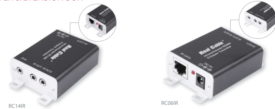
Ref. RC14IR | Infrared Extender Ref. RC06IR | Extension box (6 additional devices ir multiroom)
